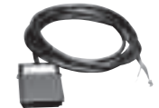
251660 – Foot switch with 3 m cord. Single pole, double throw, 15 amp @ 125-250 VAC. Wt., 0,45 kg.
