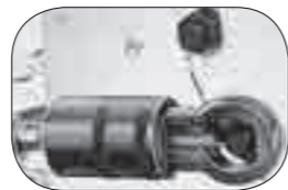
Align mark on cutter blade with scale.
